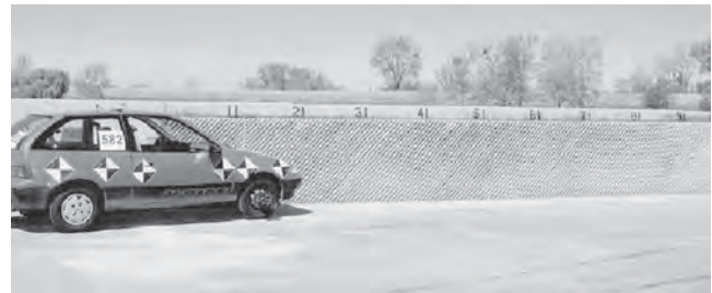
Figure 33. Caltrans single-slope barrier with fluted surface texture.
